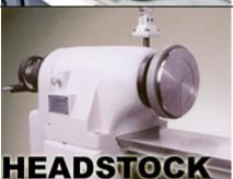
Solid one-piece enclosed headstock has high precision preloaded ball bearing spindle with 5C collet capacity. High-precision preloaded ball bearing spindle is mounted in the solid one-piece enclosed headstock, providing maximum rigidity and sustained precision. The collet seats directly in the hardened and precision ground spindle, eliminating troublesome sleeves and adapters that introduce costly inaccuracies.
