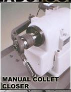
The fast lever collet closer provides faster chucking. The lever control end of the closer assembly is balanced and rides on a precision bearing. Collet tension is instantly adjustable throughout the full range from light to heavy holding power without the use of tools. The spindle handwheel is built into the end of the spindle. Entire collet closer is conveniently removed by pulling up the lock pin.
