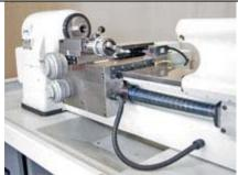
The saddle slideways are coated with Turcite-B for maximum wear resistance. The cross slideways have hardened and ground tool steel inserts for smooth accurate movement.
